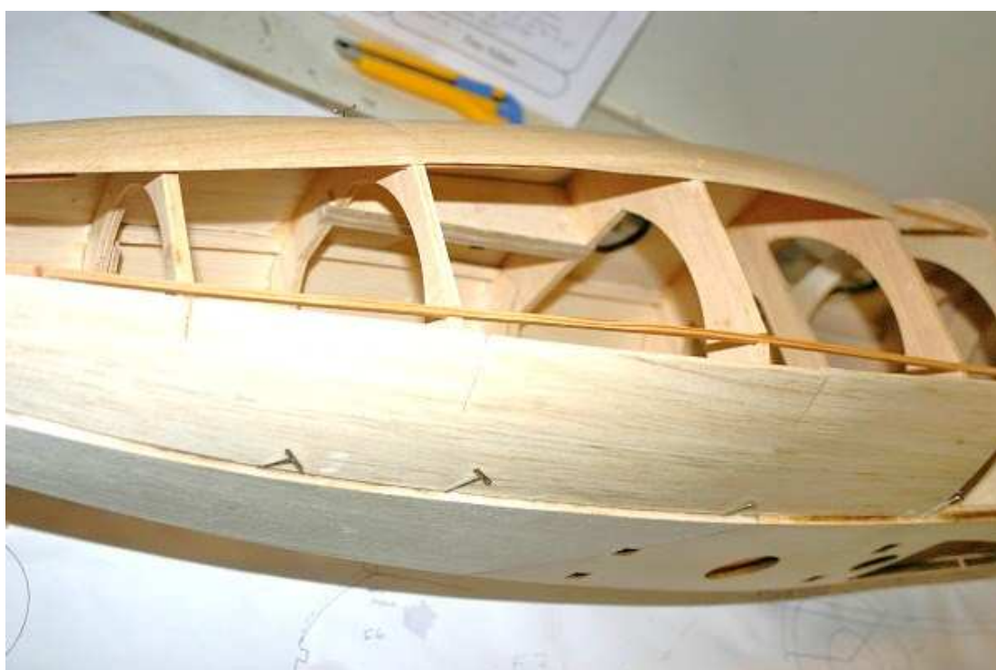
Sheeting the lower rear section
