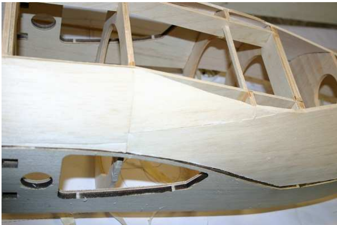
Sheeting the upper rear section. Note top 3mm stringers
