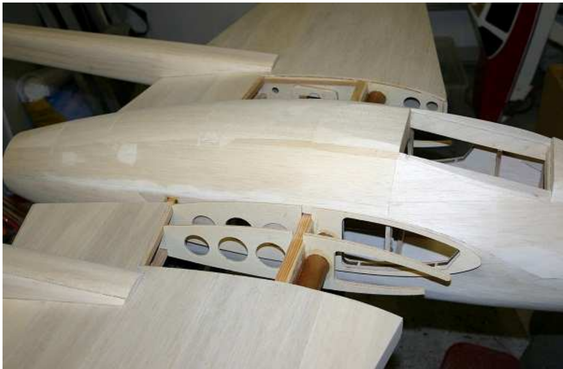
Attaching the wings. Use the booms & tailplane to 'square' the wing
