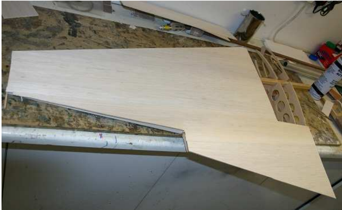
Sheeting the wings leaving section open
