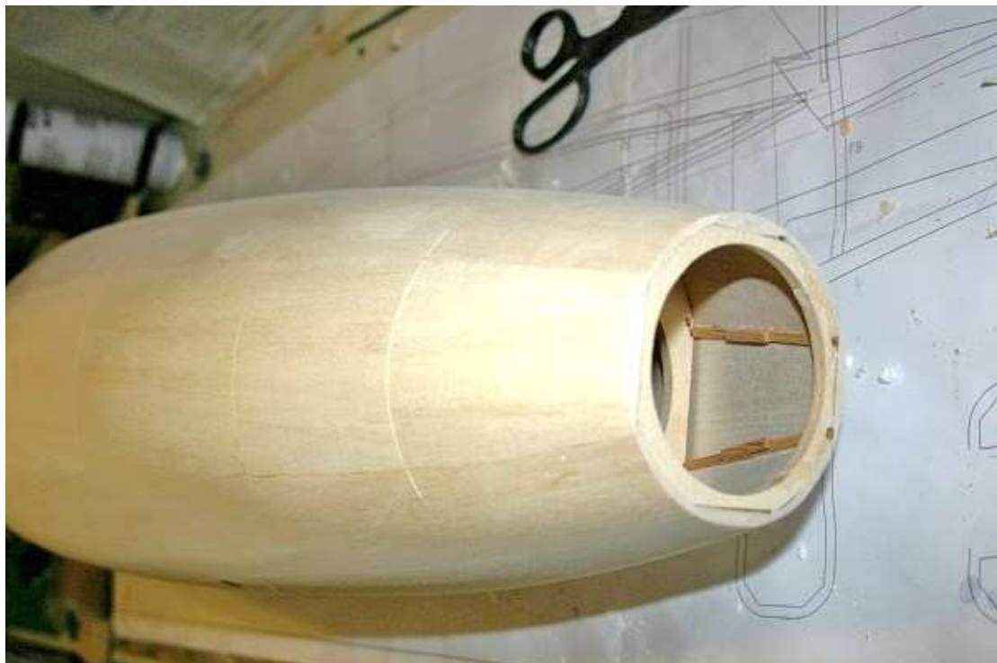
Shape to a smooth flowing 'cigar' shape using a razor plane and sand paper
