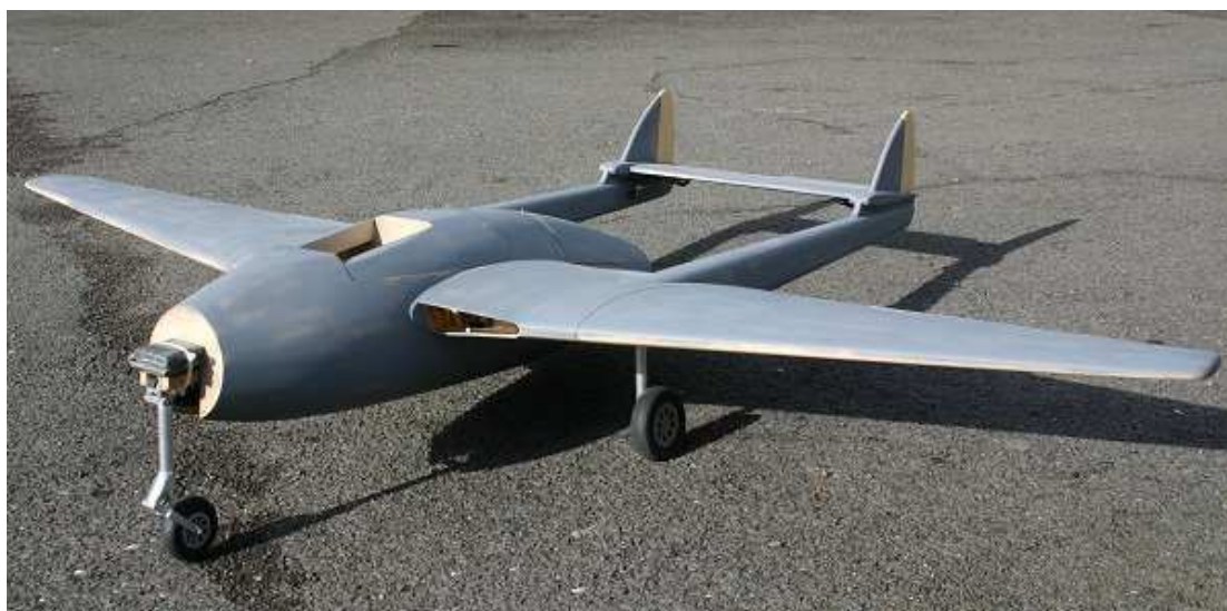
The glass cloth epoxy covered model
