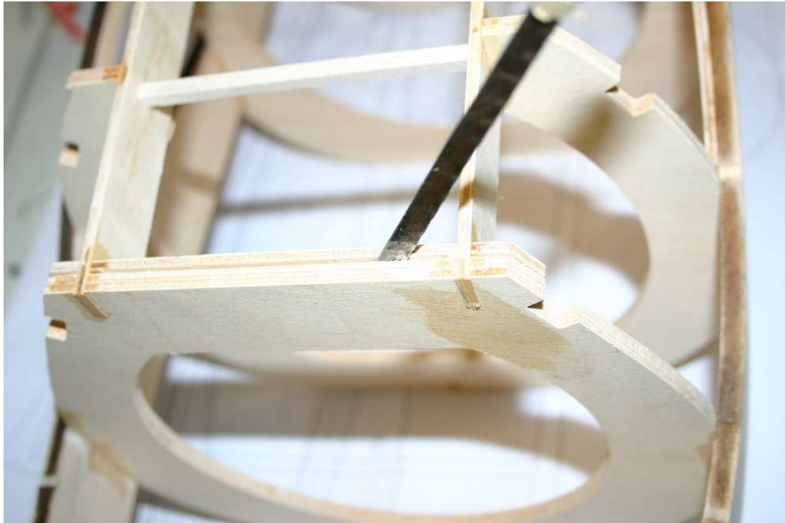
Gap between F3 & F3a to allow hacksaw blade to slid through
