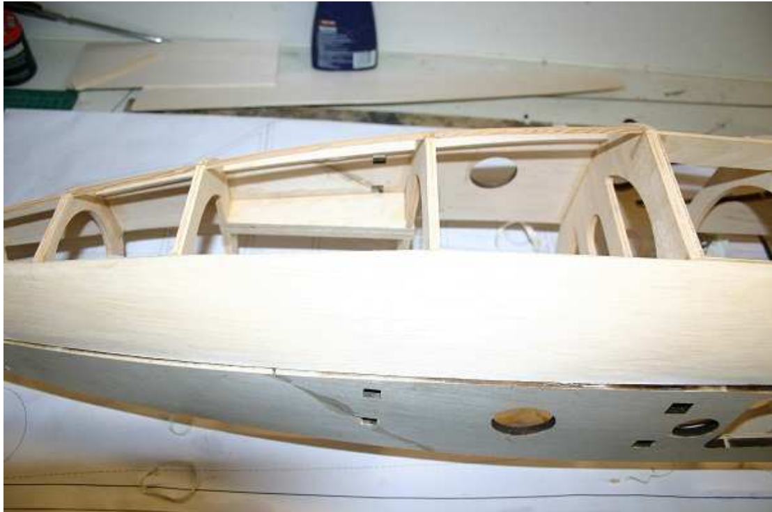
Sheeting the upper rear section. Note top 3mm stringers
