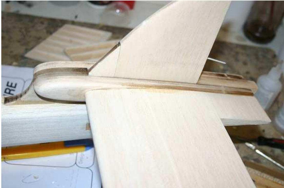
Fit the tailplane to the booms
