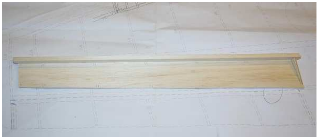
Making up the aileron
