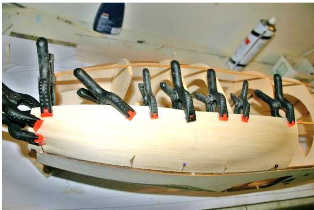
Sheeting the lower front section
